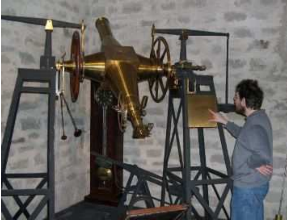
Figure 30. Cauchoix passage instrument built in 1826 which was located the Western meridian room. (© A. Heck)
