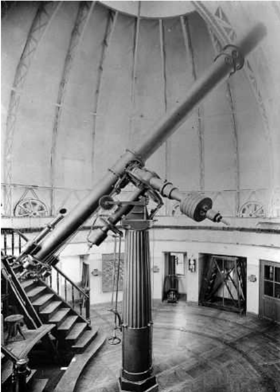
Figure 34. The Large Refractor in the twenties (Esclangon 1926). The movable stairs visible on the right are still existing. The central part can be raised and lowered to position at best the observer. (© Obs. Astron. Strasbourg)
