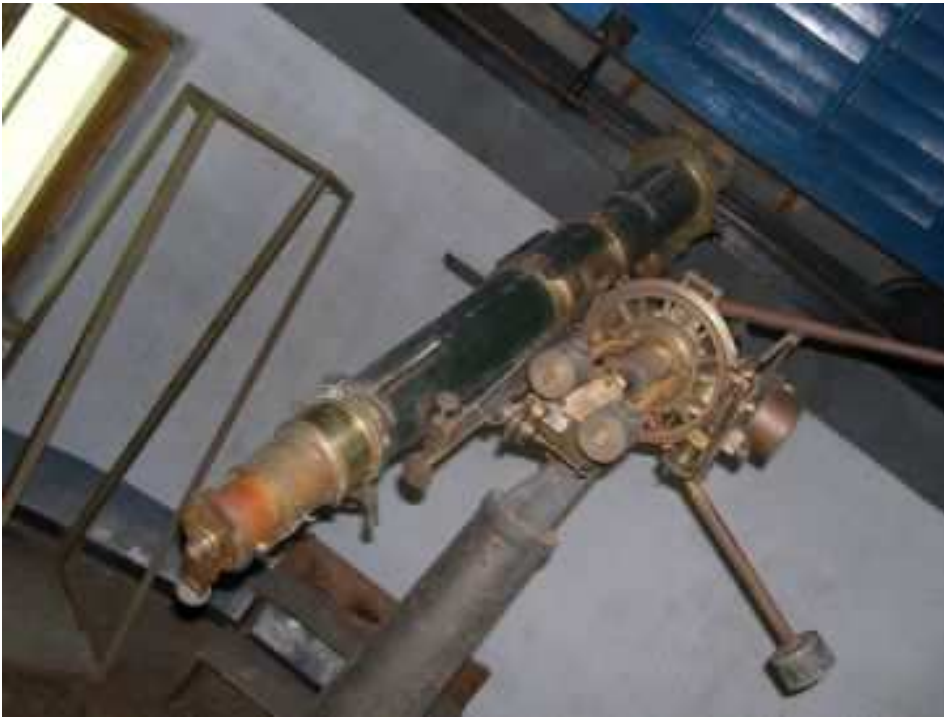
Figure 31. The 76mm heliometer, a venerable traveller that was part of expeditions (Kerguelen and Argentina) to observe transits of Venus in the second half of the 19 th century. (© A. Heck)
