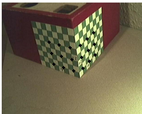
Figure 2: Calibration object. The calibration object consists of two perpendicular planes. On the planes square tiles are depicted (the sides of the tiles are 1cm). A convenient world coordinate frame is graphically overlaid on the image. The retina coordinates together with the corresponding 3D coordinates of the points indicated with a '+' are available in the file CV3_calibrationpoints.mat .
