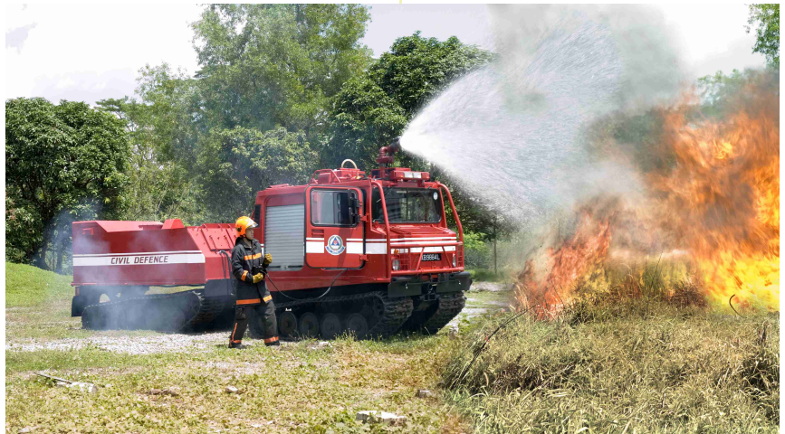
The Tracked Fire-fighting Vehicle is developed to better tackle vegetation fires.
