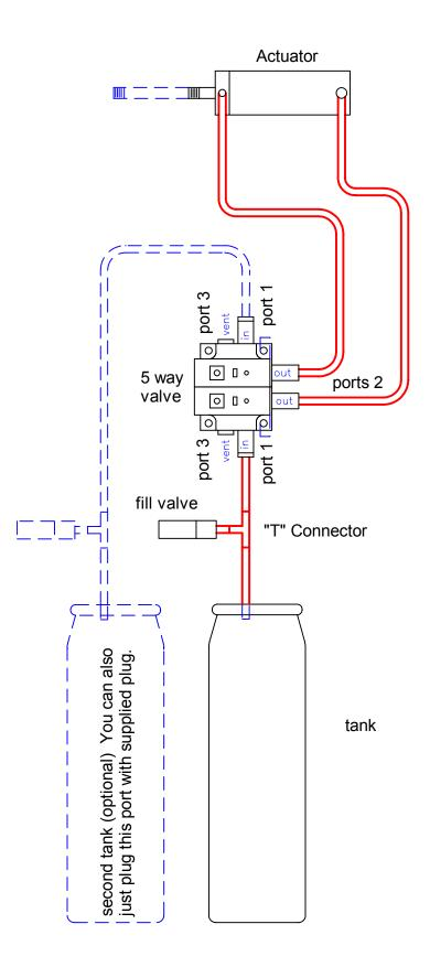
Set up for single acting cyclinders. (Cylinder powered in one direction only using gravity or spring return.)
