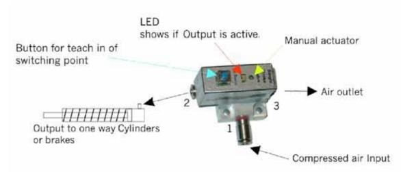
3 way valves are for faster actuation powered in a single direction using a spring, elastic, or gravity powered return. This valves only electrical connection is directly to the receiver via Futaba J connector. It replaces the servo, linkage and slow mechanical valve in most R/C pneumatic systems.
