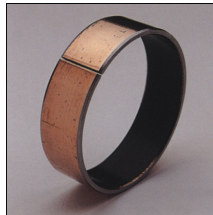
Figure 3. A composite low-friction synthetic polymer, deposited on a bronze substrate for rigidity, provides the load-bearing surface of a 45-mm-diameter bushing. (Courtesy of American Honda Motor Co. Inc.)
