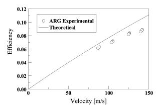
Fig. 4. Illustrating velocity-dependent efficiency for a one-turn augmented railgun.
