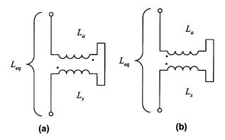
Fig. 2. The two electrical connections possible with helical gun geometry showing (a) additive magnetic fields and (b) subtractive magnetic fields.
