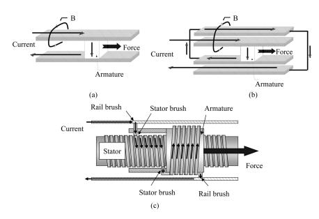
Fig. 1. Constant gradient EML geometry of the (a) conventional railgun, (b) augmented railgun, and (c) helical gun.
