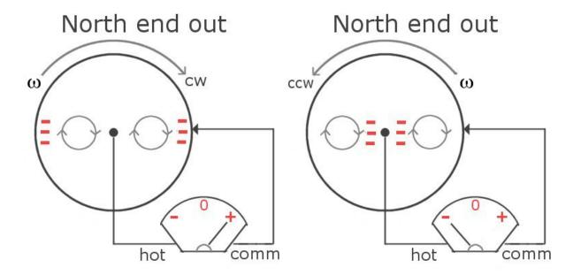
When Faraday originally performed this experiment he observed no induced EMF when the circuit was rotated with the magnet, demonstrating that the EMF indeed arises from the transformation of the reference frames.
