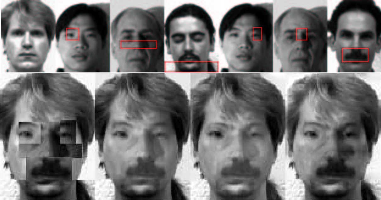
Fig. 6. A police application for generating composite portraits. The top panel shows the image parts used in the composition. The bottom panel shows, from left to right, the results of pasting the original parts, GIST1 under \ell_1 , GIST1 under \ell_2 and pyramid blending in the gradient domain. Note the discontinuities in the eyebrows.
