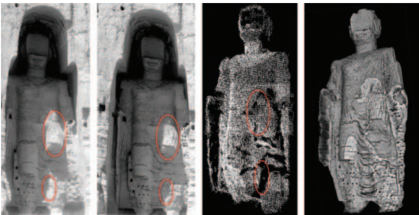
FIG. 18. Left: Two original metric images of the Great Buddha (part). Centre: 3D point cloud generated by automatic matching on the metric images. Right: Textured 3D model.
