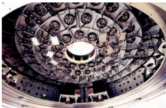
Figure 6: M1 cell seen from the back, showing the four rings of axial actuators.
