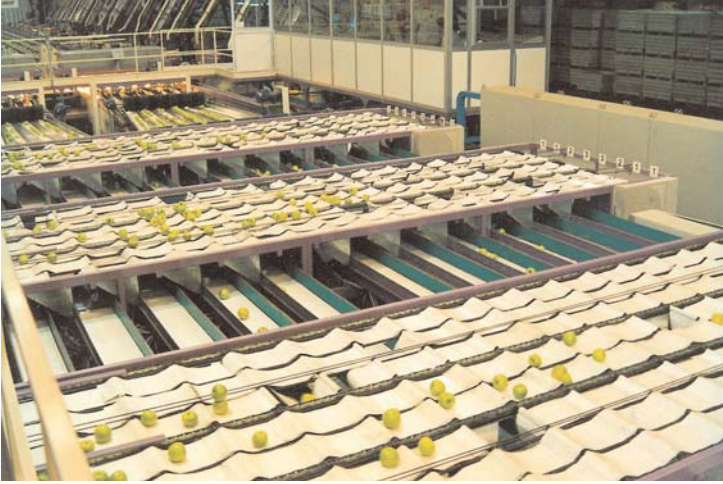
Figure 36: Sizing by weight. Individual trays deposit fruit on the corresponding conveyor belt.
