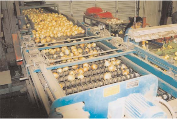
Figure 34: Sizing using rollers with increased space between them.
