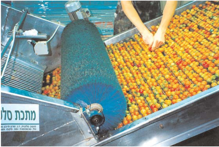
Figure 32: Brushing and hand removal of damaged fruits before grading (photograph: S. Horvitz, INTA E.E.A. Balcarce).
