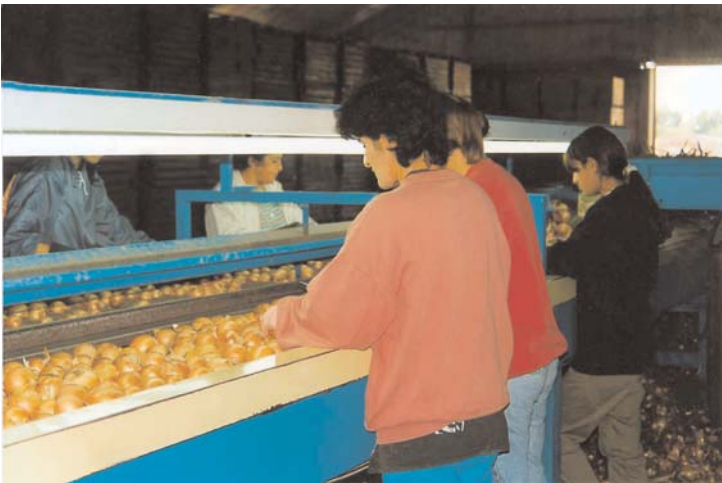
Figure 25: Lighting at eye level causes blinding and eye fatigue. Lighting fixtures should also be covered to prevent glass shattering over produce if broken.
