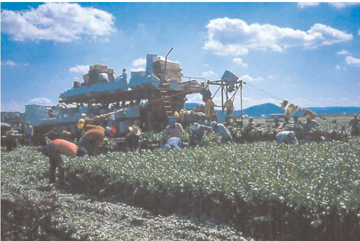
Figure 23: Mobile packing shed for market preparation of celery.
