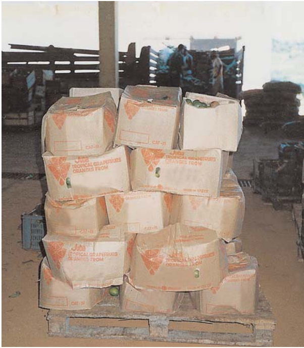
Figure 42: Weak containers or inadequate stacking patterns may collapse producing compression damages.
