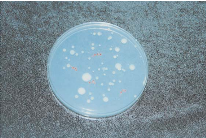
Figure 62: The total plate count of aerobic colonies on a growing media gives an idea of the degree of contamination.
