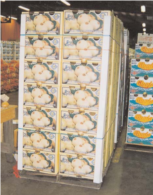
Figure 47: Pallet stabilization using corner posts and strapping.
