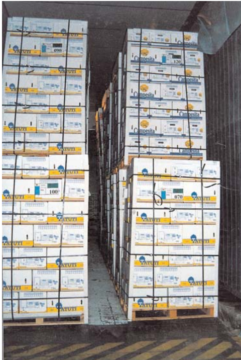
Figure 55: Inside a forced-air precooling facility. Pallets are arranged to form an aisle. Tops are covered with a canvas leaving both sides exposed to cold air. Air from the plenum tunnel is removed creating a negative pressure that forces cold air to pass through the load.
