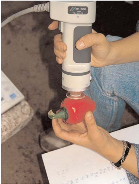
Figure 7: Objective colour measurement with a colorimeter.
