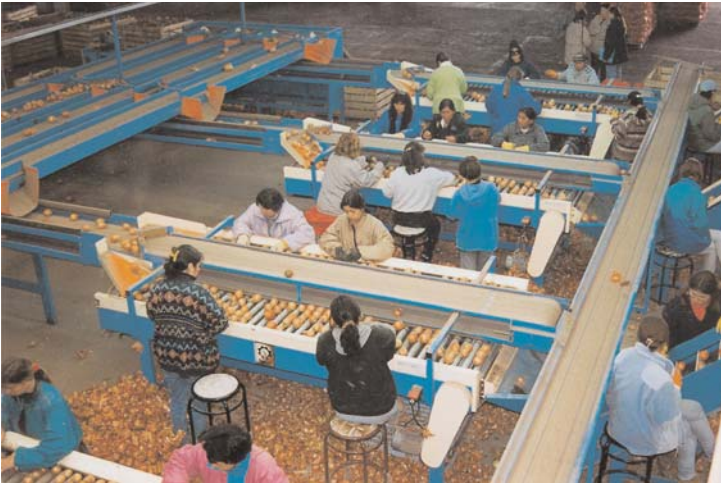
Figure 38: Dynamic quality grading system. Sized onion bulbs continuously flow on inspection tables where defective products are removed. Final inspection is performed before bagging (right-hand side).
