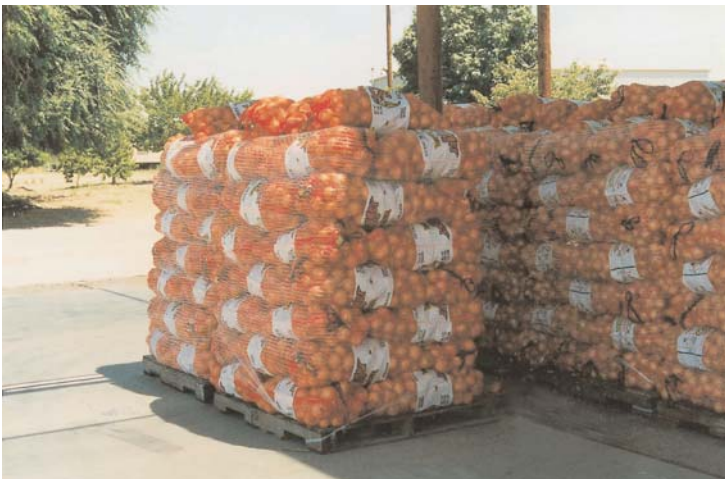
Figure 46: Pallet stabilization using mesh plastic tension netting.
