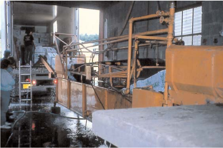
Figure 56: Hydrocooling produce and direct loading to a truck.
