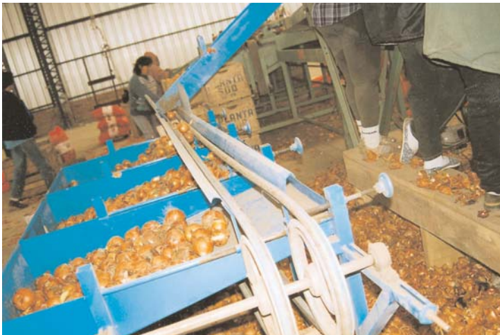
Figure 33: Sizing onion bulbs with diverging belts. The different speed of belts makes bulbs rotate besides moving forward to a point where bulb diameter equals belt separation.
