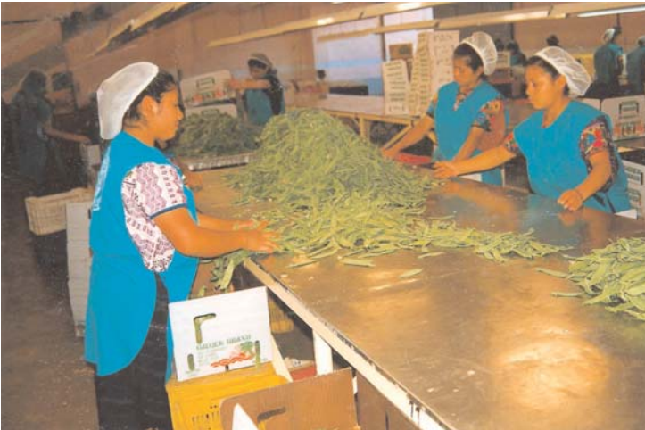
Figure 37: Static quality grading system. Product is dumped onto an inspection table where defective units are removed.
