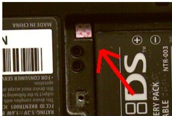
SL1 opening in a original Nintendo DS (battery cover removed, sticker left on)
