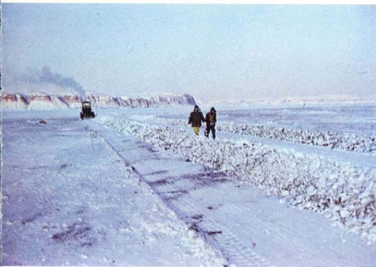
Road grader windrowing the snow in the crash area.
