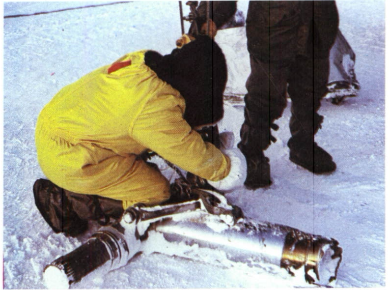
Landing gear being prepared for removal from the sea ice.
