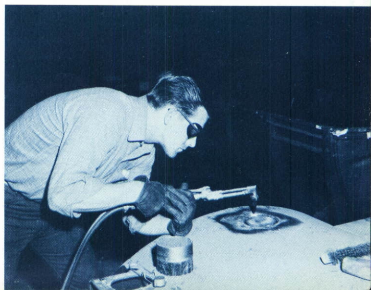
Danish construction worker cuts a filler pipe hole in the top of an R-4360 engine container.
