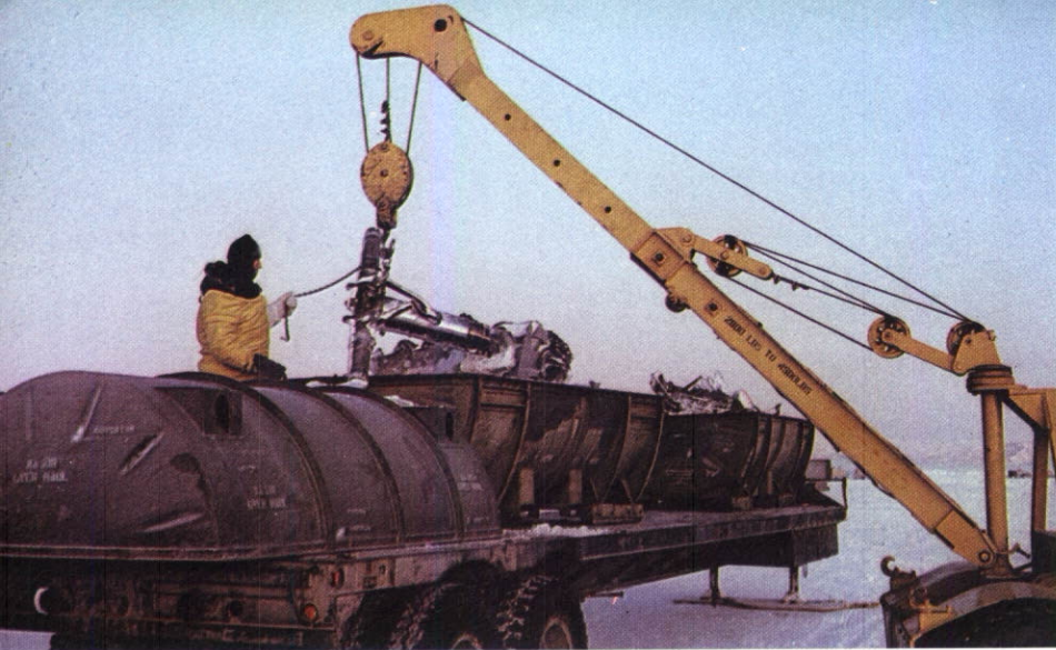
Crane hoisting engine into container.
