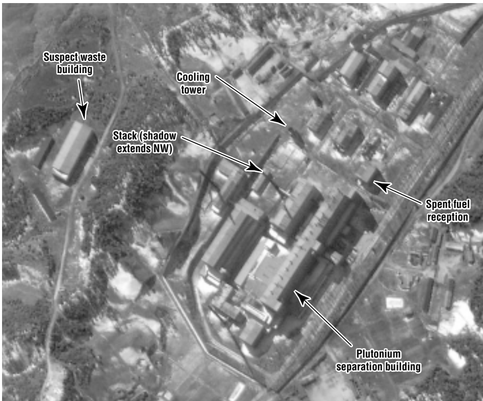
Figure 6-3. Satellite image showing the plutonium separation building and associated buildings and the suspect waste building, the so-called Building 500 where nuclear waste from undeclared reprocessing campaigns is suspected to be hidden. The waste could include 50 tons of uranium and 30 kilocuries of ^{137}\text{Cs} (used with permission from Space Imaging).
