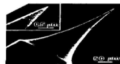
Figure 6.3 SEM micrograph showing a tip that comes rapidly to a point. This is an etched gold tip prepared by Stemmer et al. 24
