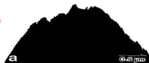
Figure 6.3 SEM micrograph showing a tip that comes rapidly to a point. This is an etched gold tip prepared by Stemmer et al. 24
