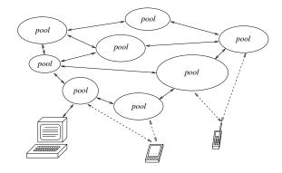
Figure 1: *The OceanStore system.* The core of the system is composed of a multitude of highly connected "pools". Clients connect to one or more pools, perhaps intermittently.
