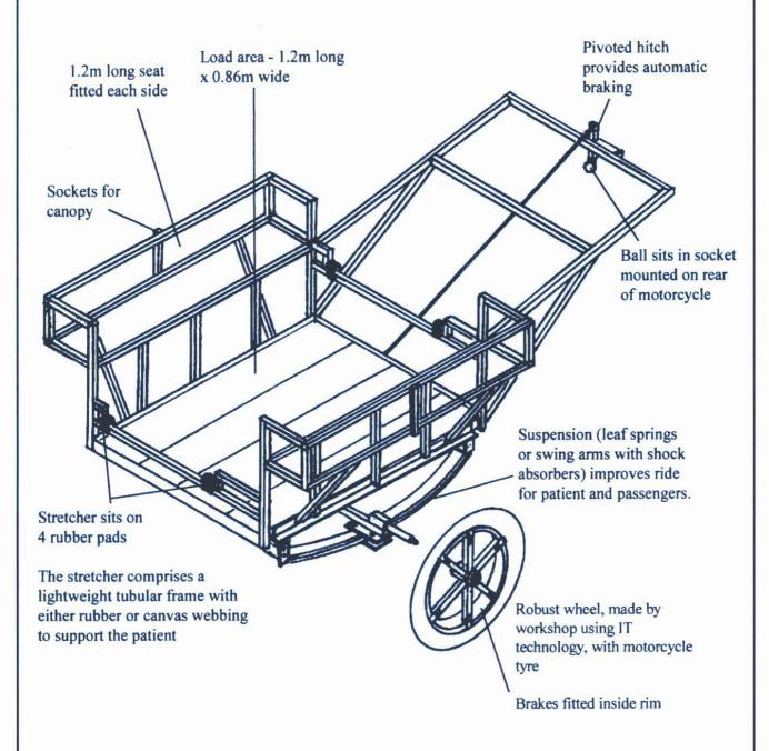
Construction: manufactured locally using commonly available materials and components. Can be
