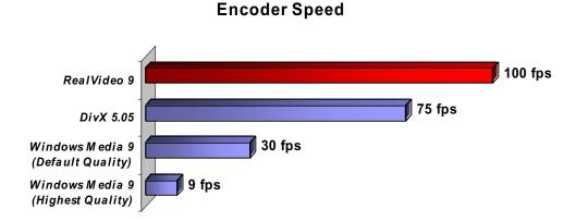
**Figure 8:** Speed while encoding the "Foreman" clip for a few video formats (speed measured encoding a 352x288 clip on a 2.2 GHz Pentium 4)
