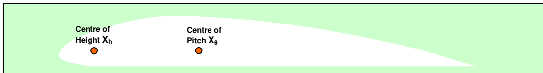
Figure 6: Relative position of aerodynamic centres for stability
