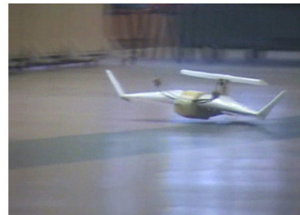
Figure 38 : Ground effect mode (Indoor hard ground testing)
