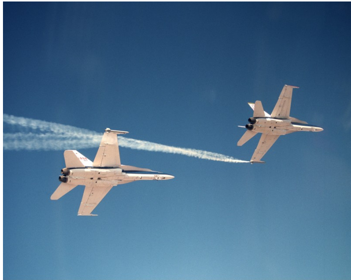
NASA Dryden Flight Research Center Photo Collection http://www.dfrc.nasa.gov/gallery/photo/index.html NASA Photo: EC01-0328-3 Date: November 9, 2001 Photo by: Carla Thomas Smoke generators show the twisting paths of wingtip vortices behind two NASA Dryden F/A-18 jets used in the Autonomous Formation Flight (AFF) program
