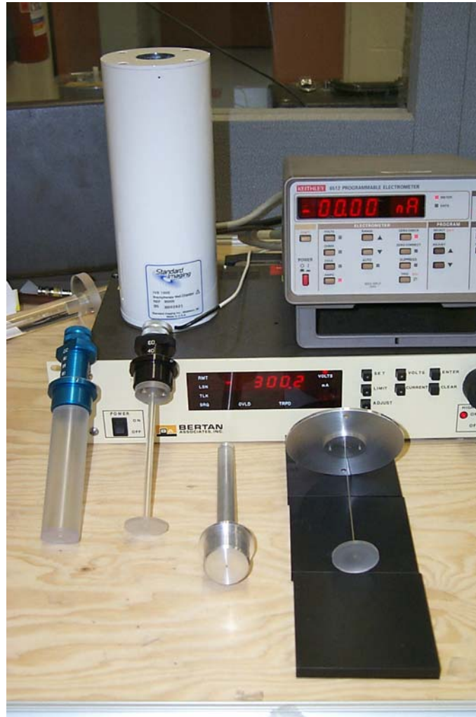
Figure A.7.2 - Well-ionization chamber for clinic use (courtesy of NIST Ionizing Radiation Division)
