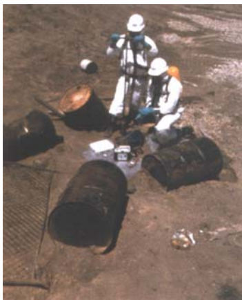
Figure B.8.1 – Soil sampling for radioactive contamination
