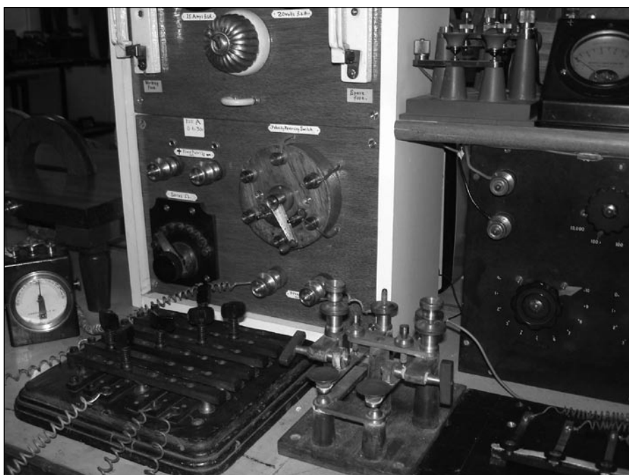
Fig. 3 The Swiss Commutator in use in the Porthcurno Instrument Room.
