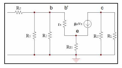
ro have little effect on the circuit operation due to their value and are removed.
