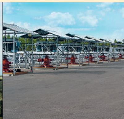
In Venezuela, subsurface pumps move heavy oil to the surface where it is upgraded for shipment to refineries.
