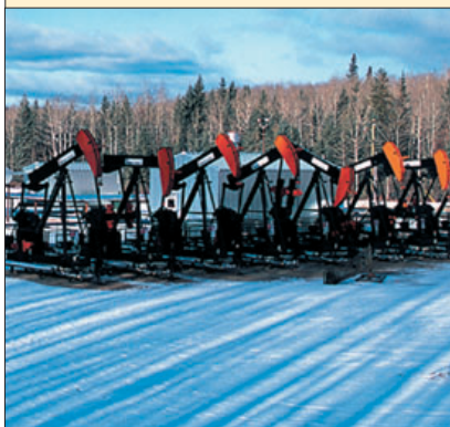
At Cold Lake in Alberta, Canada, steam is injected and heats the viscous oil. Flow is then reversed and heated oil and water are pumped to the surface.
