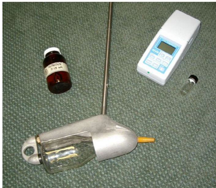
Figure 44. Photograph of the DH-48 hand-held depth integrating sampler, amber glass suspended sediment sampling bottle, the portable turbidimeter, and clear glass turbidity sample container.
