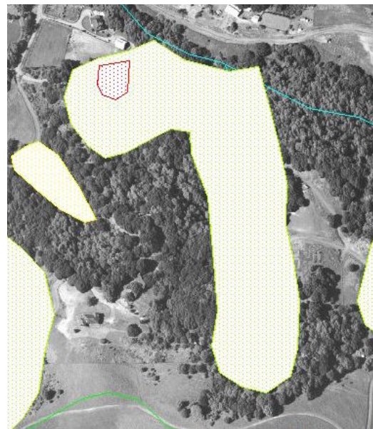
Figure 14. Example of a typical Holocene landslide with a younger active landslide mapped within it.
