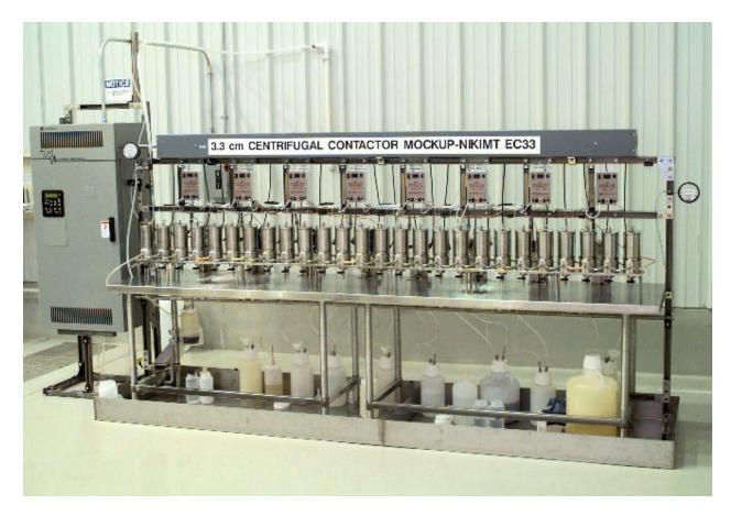
Fig. 1. 3.3-cm centrifugal contactor pilot plant.
