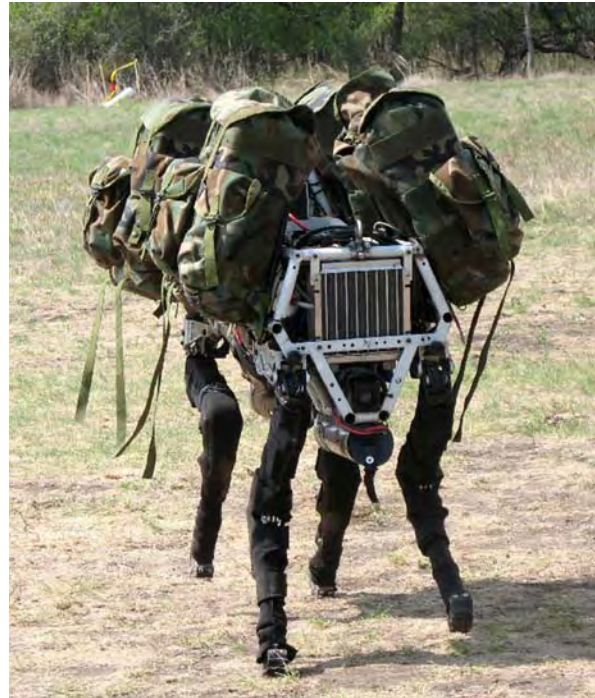
Figure 35: Bio-inspired “Big Dog” quadruped robot is being developed as a “mule” that can traverse difficult terrain.
