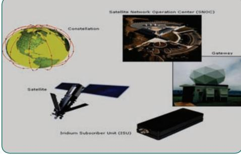
at an altitude of 780 km and 86.4° inclination. The Iridium network is designed to operate in the L-band of 1616 to 1626.5 MHz for ground user links; in the Ka-band of 19.4 to 19.6 GHz and 29.1 to 29.3 GHz for gateway down- and up-links; and in the Ka-band of 23.18 to 23.38 GHz for Inter-Satellite Links (ISL). The exact L-band frequencies used depend on local regulating authorities and issued licenses in any particular region.
