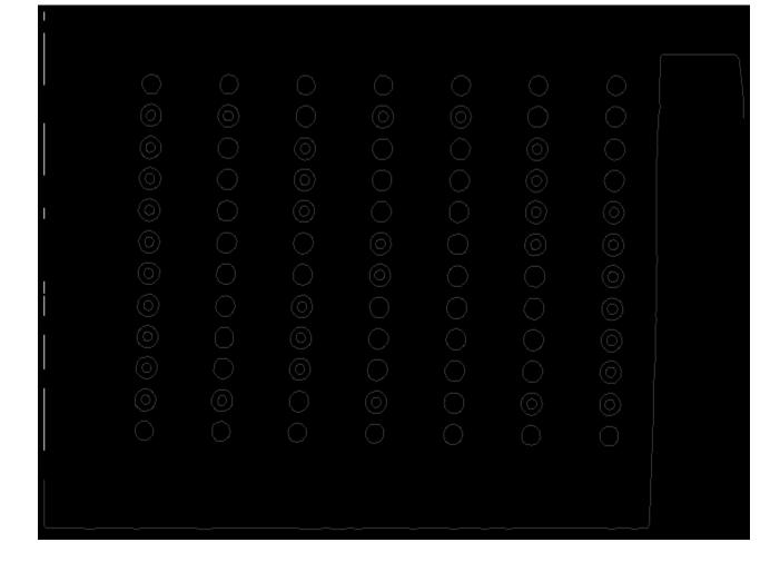
After the automated tuning and finding the edges, the analysis algorithm looks for the filled-in rows of bubbles at the top and bottom of the image. Then, the bubbles between the top and bottom rows are analyzed for a user mark.
