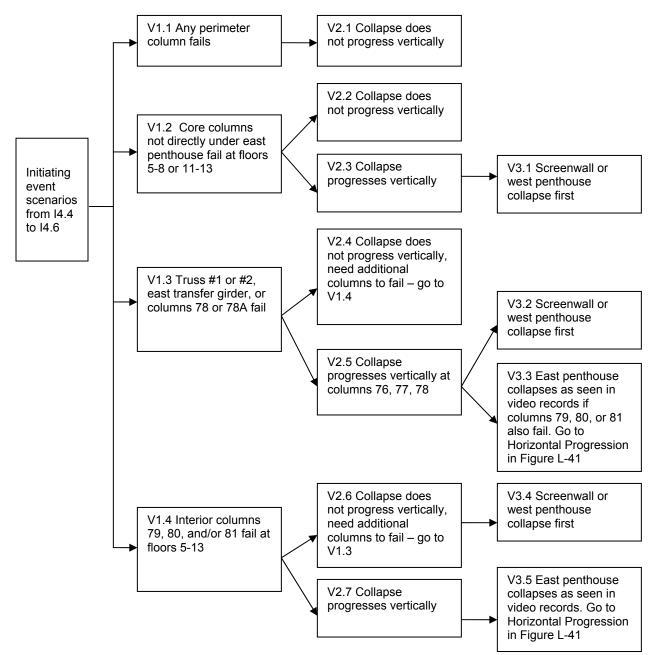
Figure L-40. Vertical collapse progression scenarios.
