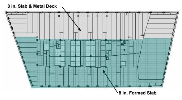
Figure L-13. Floor 7 plan.
