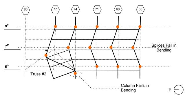
Figure L–49. Horizontal progression mechanism for truss #2 failure.
