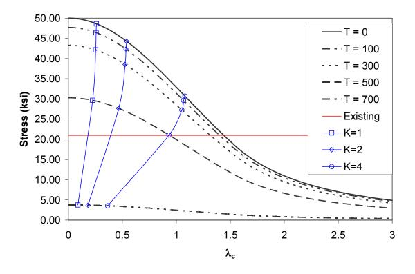
Figure L–37. Column 79 capacity versus temperature and unbraced length K.
