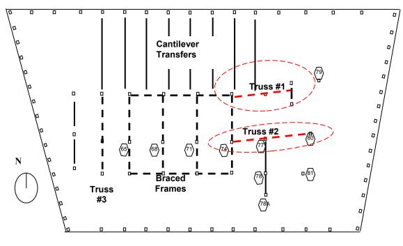
Figure L–47. Transfer components between Floors 5 and 7.
