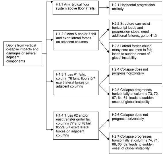
Figure L-46. Horizontal collapse progression scenarios.
