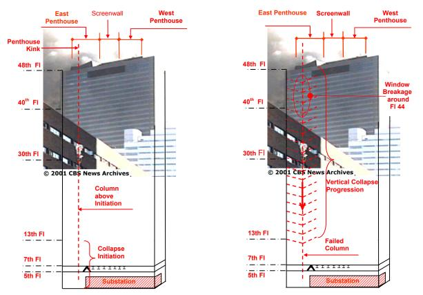
Figure L-33. Collapse initiation and vertical progression on the east side of WTC 7.
