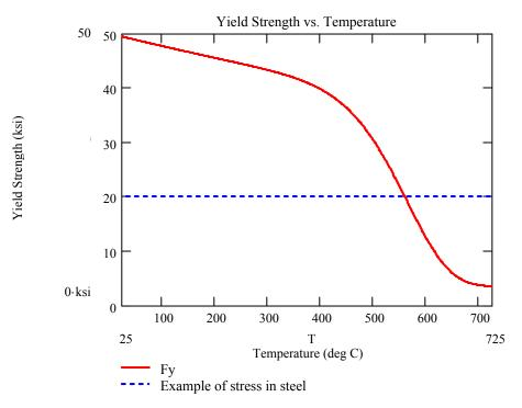
Figure L–39. Steel strength versus temperature.
