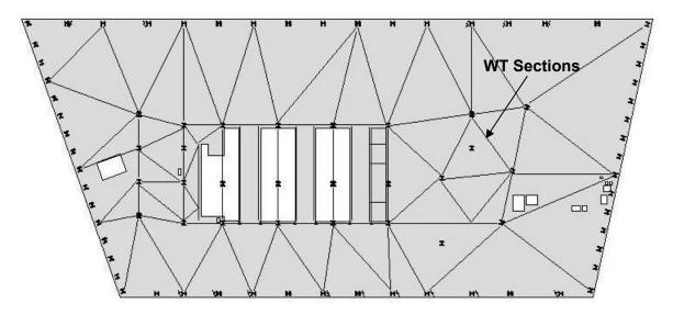
Figure L–11. Floor 5 diaphragm plan.
