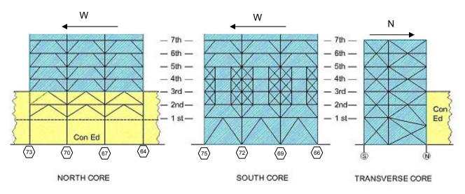
Figure L-20. Core lateral system.
