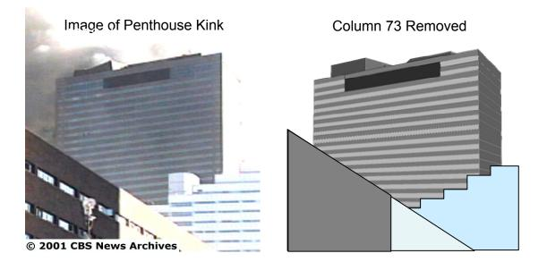
Figure L–41. Geometry changes for removal of column 73.
