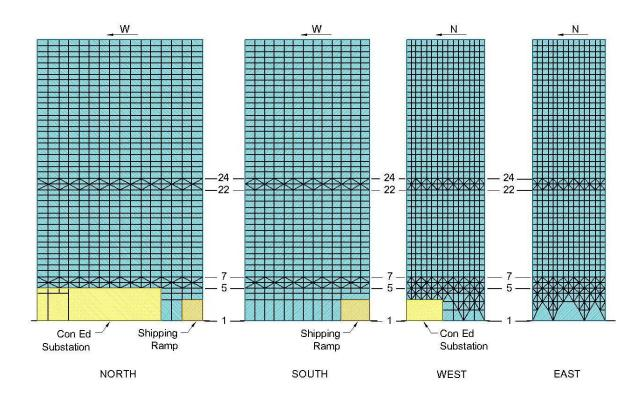
Figure L–19. Perimeter lateral system elevations.
