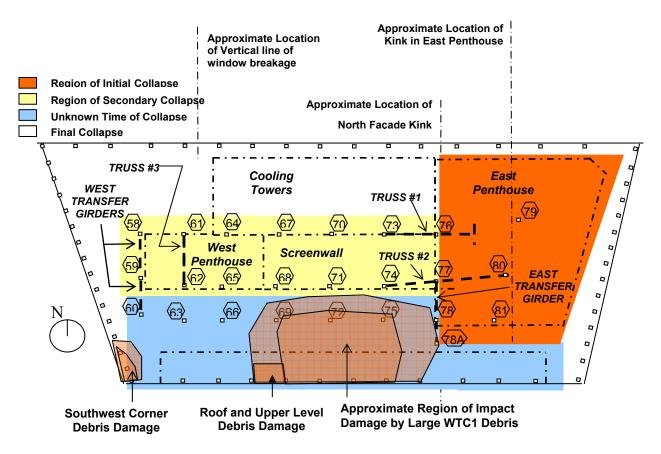
Figure L-31. Plan View of Collapse Progression.
