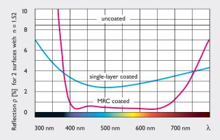
most of these filters are also available with MRC multi-layer coatings. B+W polarizing filters have different coatings, depending on the kind and on the glass diameter. The overview tables for all B+W filters on pages 62 to 64 show the kind of coating for each type and size of filter.
