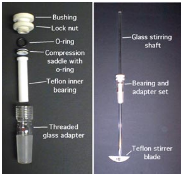
Figure 9. Left: Assembly of the bearing and adapter set. Right: Assembly of the stirring apparatus.
