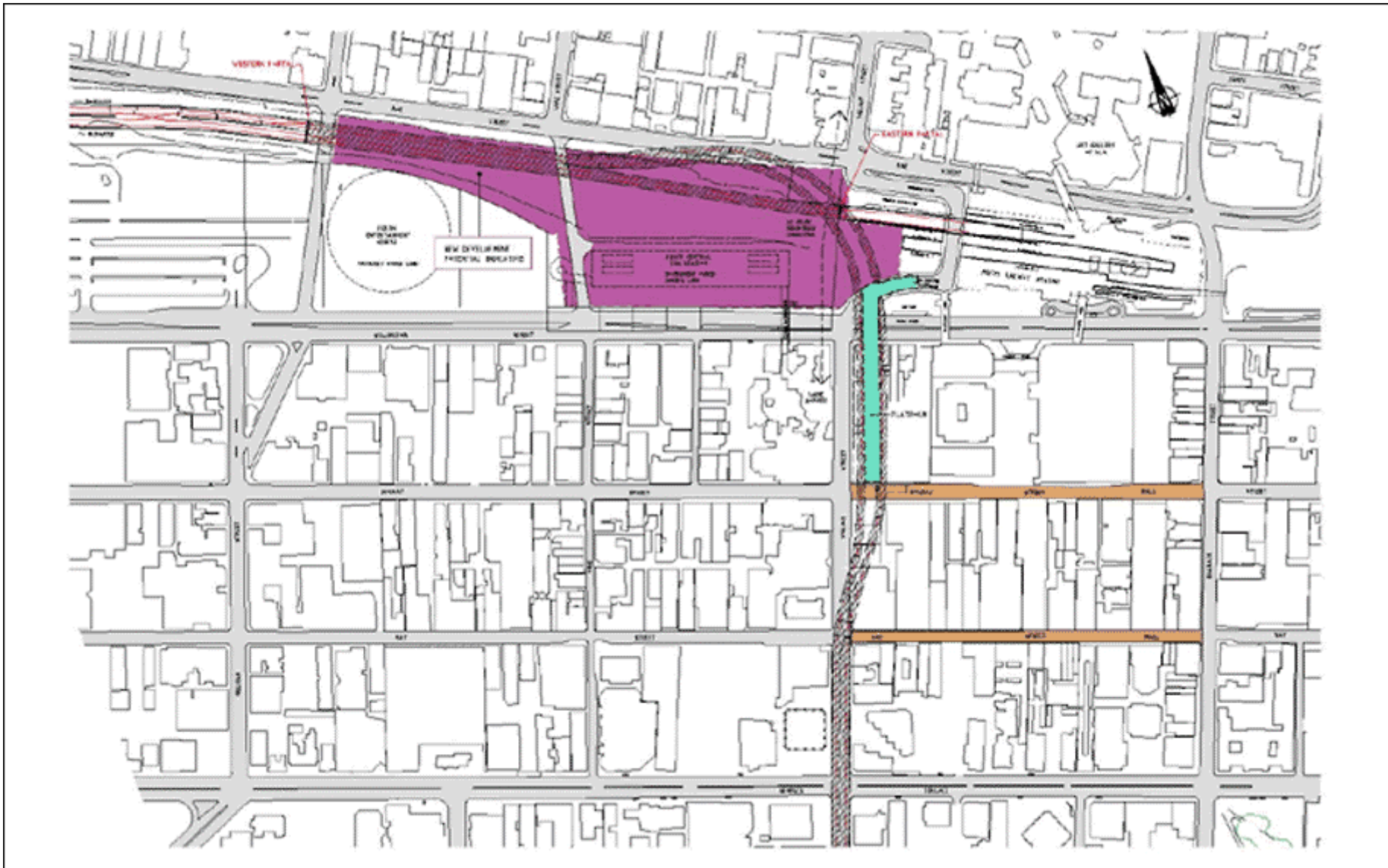
Figure 20 - Land Development Potential if the Fremantle Rail Line was Sunk to Milligan Street (Option 2)
