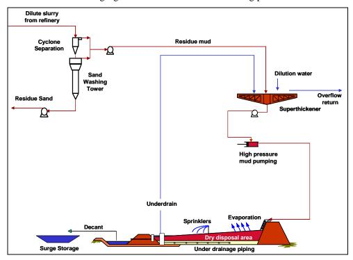
Figure 2 Schematic of the dry stacking process
