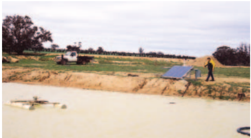
Above: A solar-powered aerator (invented by Ian Pederick) increases the efficiency of marron ponds, a profitable sideline to water harvesting.
