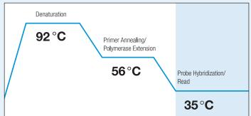
The cycling conditions for Abbott RealTime HIV-1 encompass a low temperature read cycle. This read cycle allows the probe to tolerate mismatches more effectively than a probe required to bind during the extension phase.
