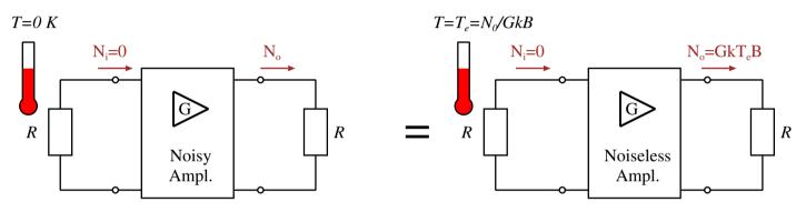
The equivalent noise temperature  $t_e$  of an amplifier is the temperature to be added to the input resistance temperature, in order to represent the noise inside the amplifier
