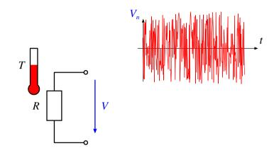
A resistor R at Temperature T generates an available noise power (matched load with R) of
