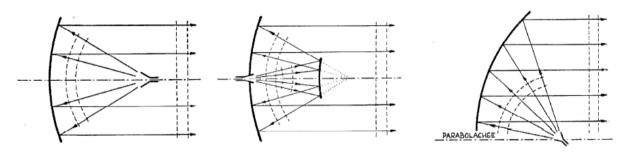
Parabolantenna: a) Parabolantenna with central feed b) Cassegrain-Antenna with secondary reflector, c)Offset-Parabolantenna
