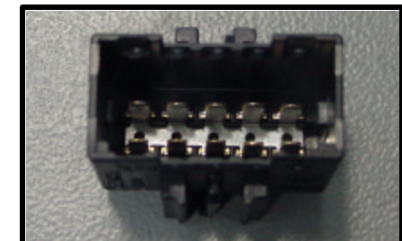
Bridge cover removed showing bridge contacts
