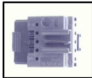
Bridge cover pulled up into 'test position' disconnecting wake-up lines
