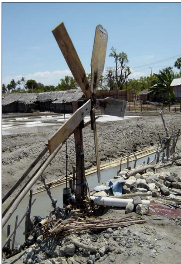
Figure 14. Small capacity wind pump (locally made; can be scaled up to handle higher pumping rates).
