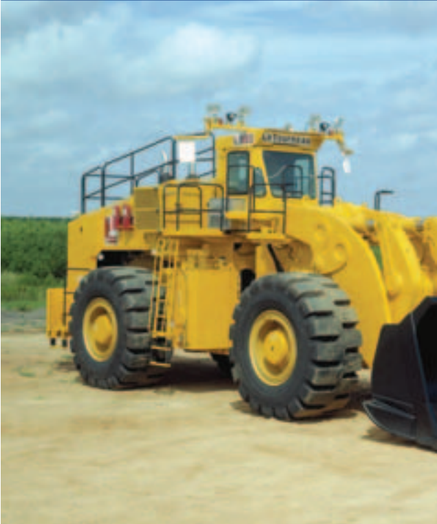
Left: the LeTourneau L-950 Pit Bull loader incorporate the company's new Switched Reluctance (SR) drive, which is somewhat like a cross between DC and AC. While this system has a number of advantages over conventional DC drive, currently it is not available on the company's larger machines
