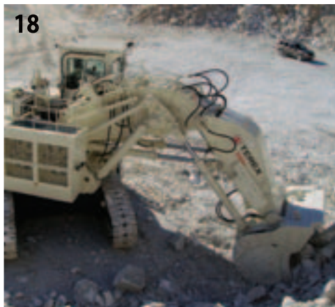
18 The 280 t Terex RH120-E is now available with either a Cummins or Caterpillar engine
