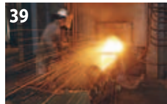
39 Matte tapping at the Fortaleza nickel smelter, Mineracao Serra da Fortaleza Ltda, Brazil
