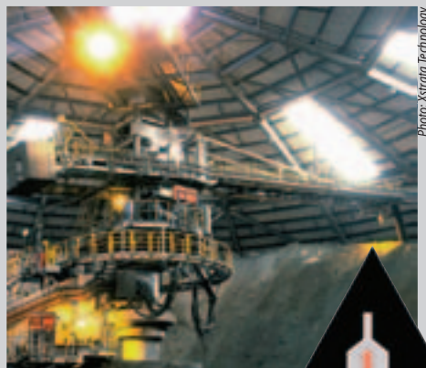
ISASmelt treats a variety of raw materials. Pictured is the stacker-blending copper concentrate
