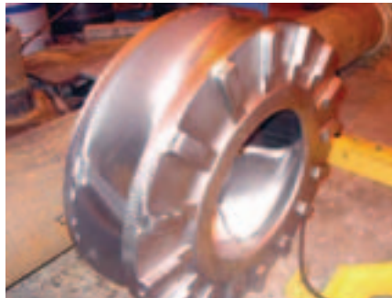
An impeller and suction liner from GIW's Slurry Diverter
