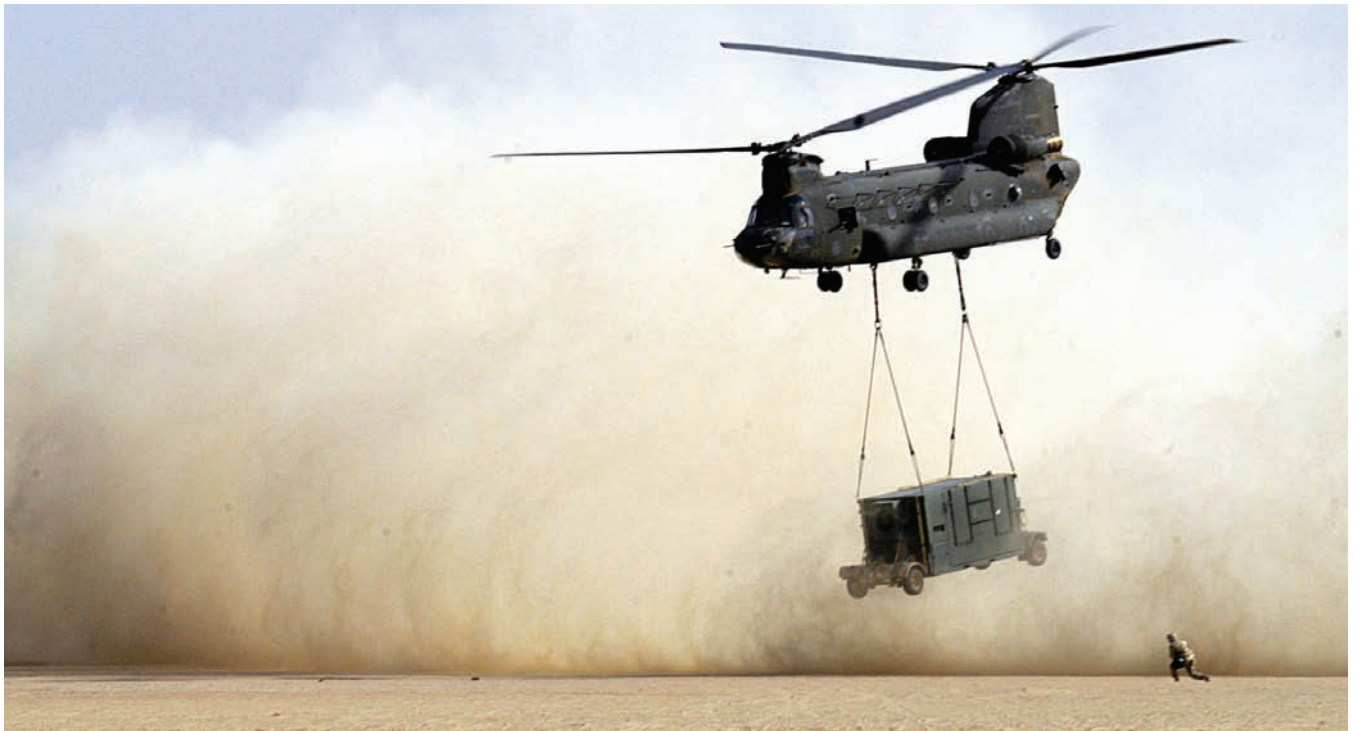
Brown-outs can easily occur during take-offs and result in about 20 percent of the accidents with damage. Here a CH-47 Chinook lifts off during a March 2003 mission with a communications container in Iraq, creating brown-out conditions that could hamper other aircraft in the area.
