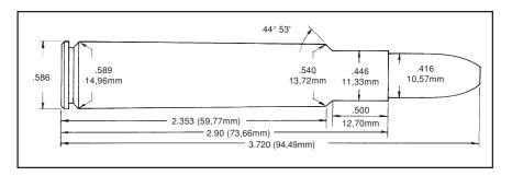
The .416 Rigby is a large case. The combination of a large case capacity and a low working pressure reduces the selection of suitable propellants drastically.
