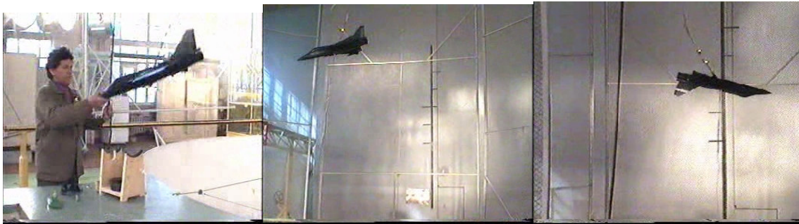
Fig-7: 1:15 Scale Model and Spin Tests Underway
