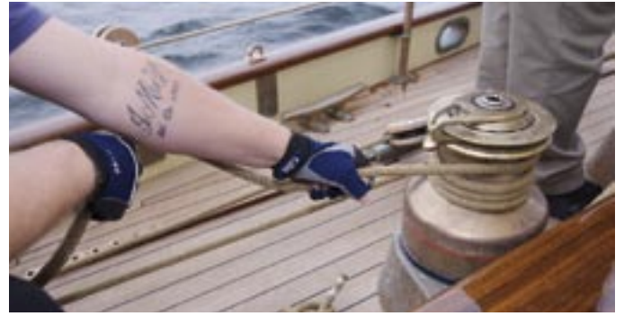
Four bronze winches control the foresail and mainsail sheets
