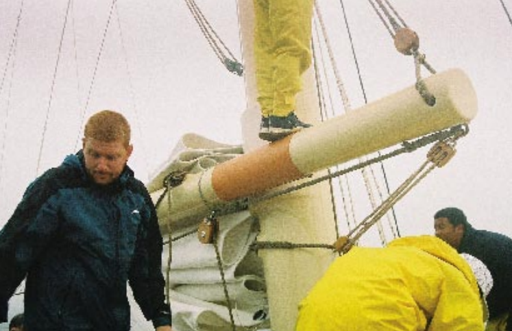
Her mizzen boom is attached to mast with ropes and blocks
