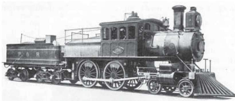
Top: 1880 Saddleback Bottom: 1883 Saddleback Saddleback engines were the first steam engines specifically designed to burn anthracite coal. These two were run on the Philadelphia and Reading Railroad.
