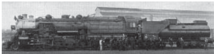
The mighty Baldwin #60000. This three cylinder demonstrator was eventually donated to the Franklin Institute in Philadelphia, where it can be seen today.
