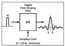
Figure 6. Converting an impulse to a raised cosine pulse by filtering.
