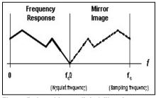
Figure 5. An arbitrary digital filter frequency response.
