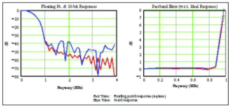
Figure 7. The frequency responses of two different versions of the raised cosine pulse-shaping filter.
