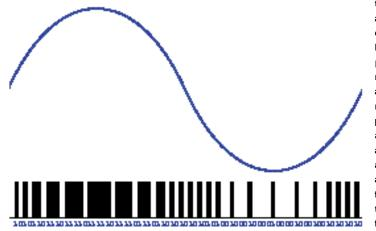
I ne resulting pulse train has some remarkable properties. Like PCM digital audio, DSD is inherently resistant to the distortion, noise, wow & flutter of recording media and transmission channels. But unlike PCM, DSD "looks" quite analog. Simple inspection of the digital pulse train tells you much about the frequency and amplitude of the waveform. And digital-to-analog conversion can be as simple as running the pulse train through an analog low-pass filter!
