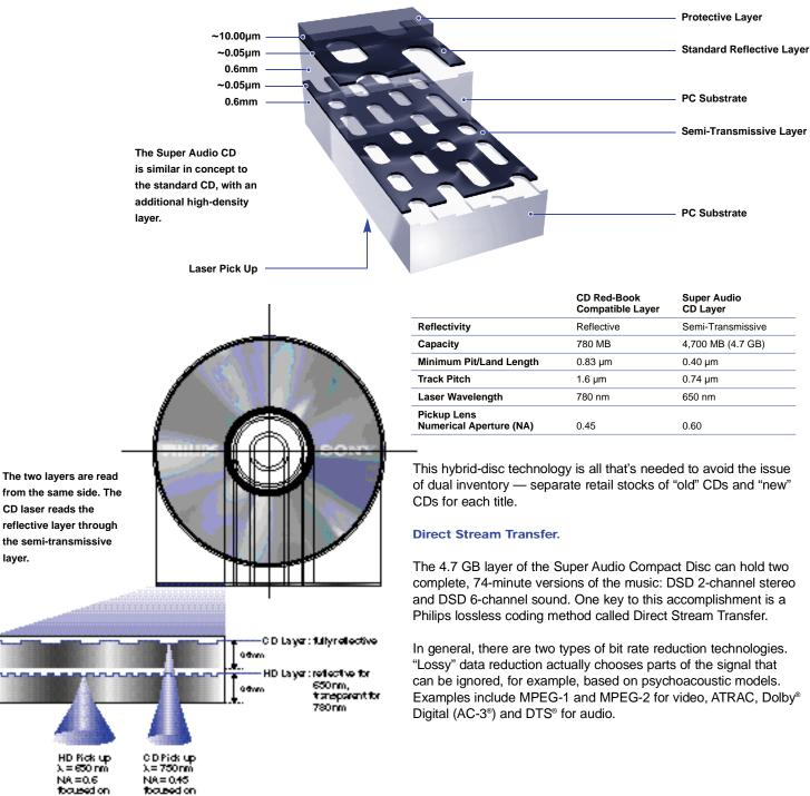
from the same side. The CD laser reads the reflective laver through the semi-transmissive layer.
