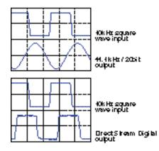
A notorious torture-test for recording systems, the 10 kHz square wave (top trace) includes component frequencies well above the audio band. The 16-bit PCM system approximates this with a 10 kHz sine wave (second to top trace). In comparison, the 1-bit Direct Stream Digital captures the wave's true shape (bottom trace).
