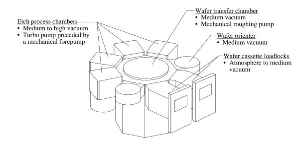
The process chamber is a controlled vacuum environment where intended chemical reactions take place under controlled conditions. Process chambers are often configured as a cluster tool.
