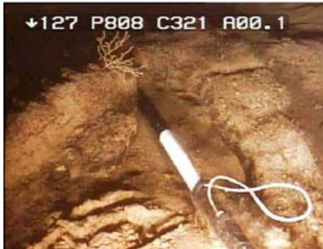
Figure 17: North anchor flukes, 1-meter scale
