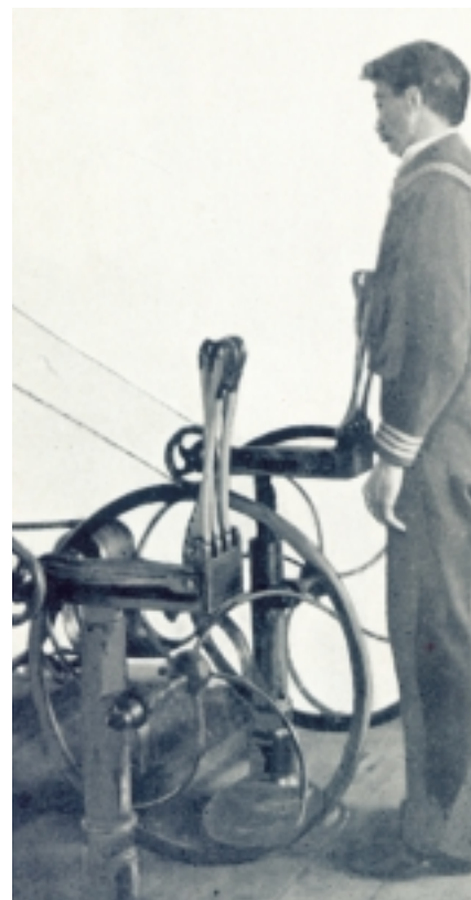
Figure 8. Beating machine with padded levers, c. 1890
