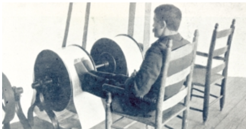
Figure 9. Revolving ribbed cylinder for friction of the feet; apron prevented wear on socks and build up of static electricity, c. 1890
